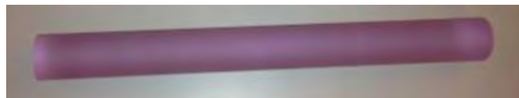
LG-760 rod (2wt% Nd 3+ , ca. Ø25x250 mm 3 ) double side AR coated with LIDT > 50 J/cm 2 (10 ns, 1064nm)
