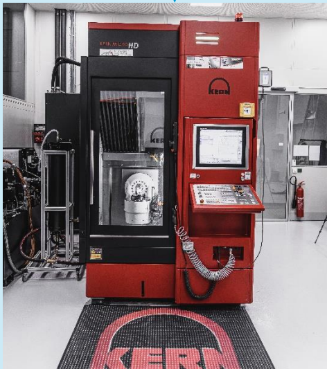
5-axis machining centre Kern-Microtechnik «Micro HD» (Part accuracy <math>< 2 \mu\text{m}</math>)
