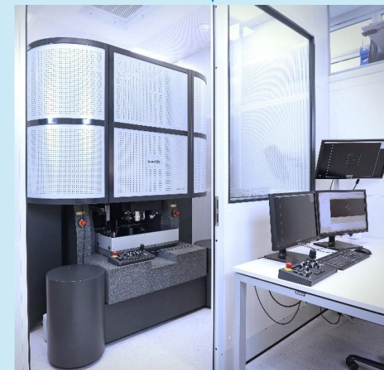
Multisensor coordinate measuring machine WERTH «VideoCheck UA» (measurement uncertainties <math>< 0.1 \mu\text{m}</math>)
