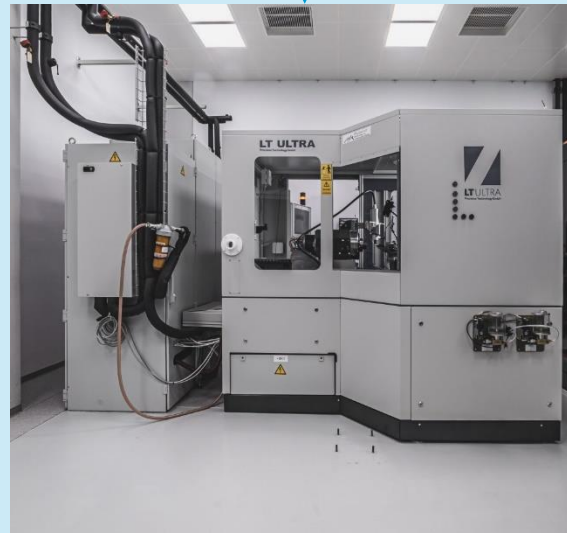
Ultra-precision turning LT-Ultra «MTC 650 UP» (Part accuracy <math>< 0.1 \mu\text{m}</math>)
