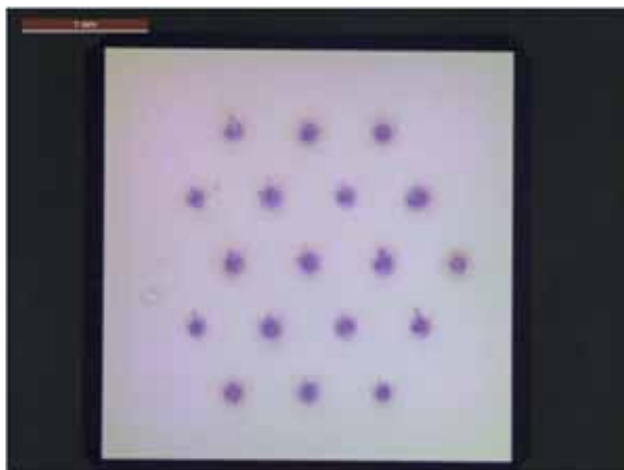
Above: Matrix of LIDT measurement sites used in a ramp-test on a 3.6 mm x 3.6 mm laser crystal
