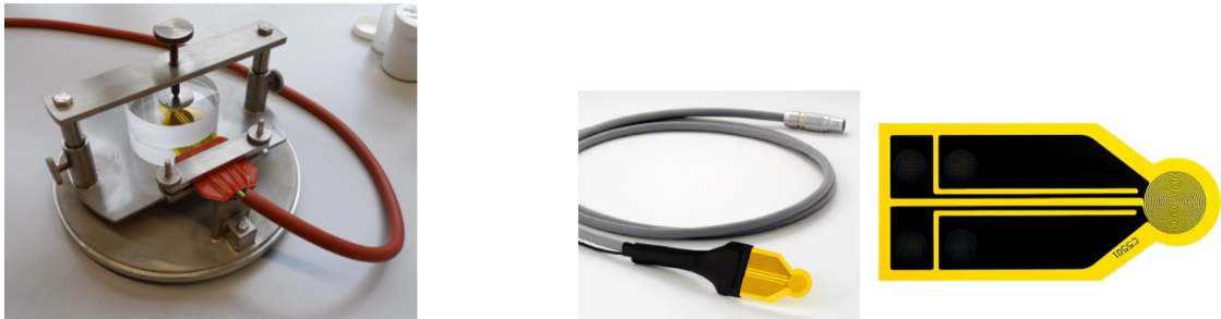
Figure 4: Hot disk sensor. On the left you can see the sensor clamped between two samples, on the right detailed images of the sensor.
